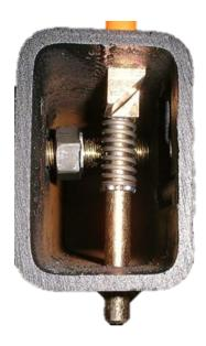
The Plunger Pin runs vertically through the middle of the frame.
