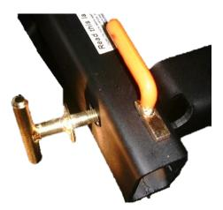
The latch with the orange handle on top is the Plunger Pin.
