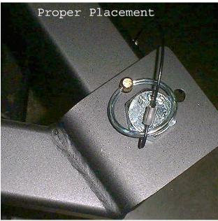
**Open Position Pin Placement**. When the frame is in the open position, the "front" hole will not allow the pin to pass through (shown in left below). Proper pin placement should be in the "back" hole (shown in right below). The frame will need to be at almost exactly 90 degrees for the pin to insert properly into the "back" hole.
